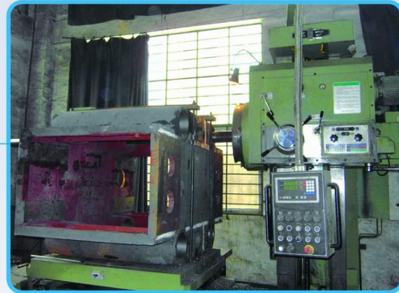
2 采用数控镗床加工柱孔、主轴箱等，有效保证同心度的加工精度，提高产品稳定性。 Sliding ways of up/down system are quantity proceed by completely new grinding machine, for the purse of high precision and quality.
