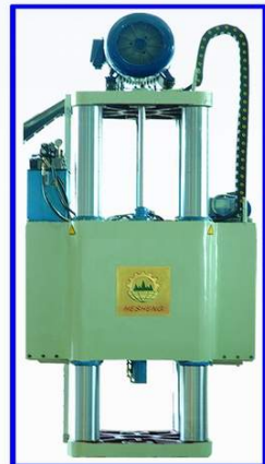
升降导柱采用四根表面经精度硬铬处理的圆钢，有间隙小，整体刚性好，切割时晃动小，使用寿命长等优点。 Up/Down sliding ways are made up of chrome-plated round steel to minimize cutting clearance and trembling, and to endure the using life of machine.
