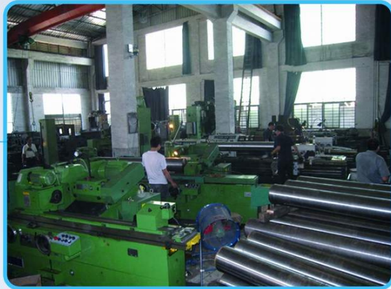
1 采用全新磨床批量加工导柱，加工精度高，质量有保证。 Use CNC boring lathe to process the hole of sliding column and headstock, to ensure the concentric and stability.
