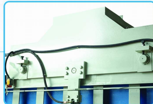
8 横梁两端架采用液压锁紧装置，可进一步提高机台切割的稳定性，使板材平整度和刀头使用寿命都有显著提高。 "Hydraulic locking device" which using on the end frame of crossbeam, can further improve the stability of cutting, and markedly improve flatness of cutting and the using-life of blade tools. (*选配 Alternative)
