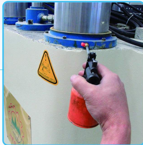
4 导柱升降采用润滑油来润滑，每一星期添加一次，大大减少维护次数。 Up/Down column movements are lubricated by lubricating oil, which should be added once a week, it will reducing the machine maintenance frequency.
